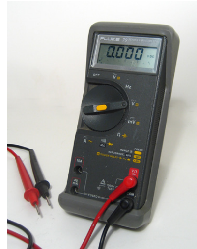
Measure defroster electrical properties to help in troubleshooting.
